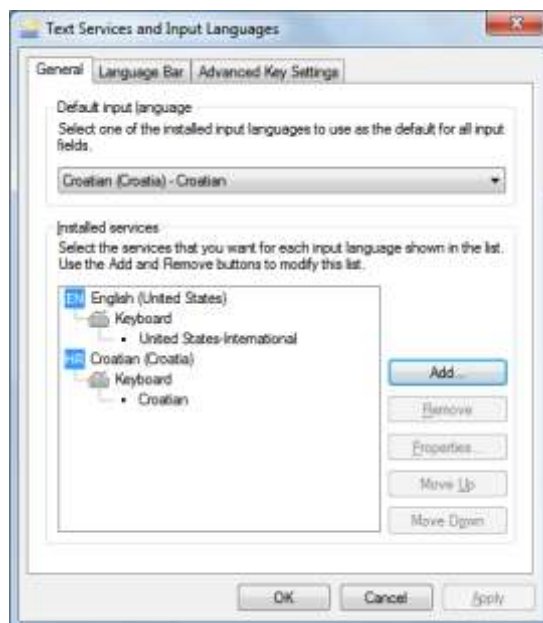
Sl. 13 Odjeljak Instalirani servisi (Installed services)
